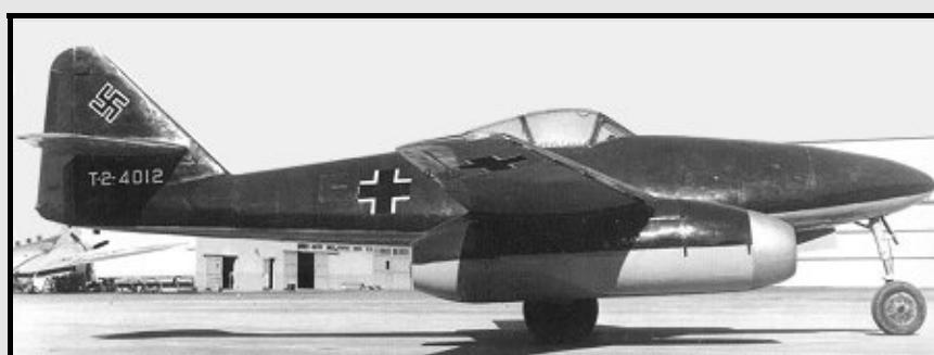
The world's first operational jet fighter, the Me-262 Schwalbe, was powered by two Junkers Jumo 004 B turbine engines and had sleekly swept wings and a powerful armament of four 30-mm cannons. With a top speed of approximately 869.4 kph (540 mph), the 262 was
