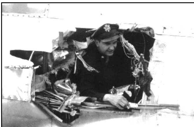
Damage from flak on 1Lt Miller's B-17 #42-97329 Flak Hack. It was hit by an 88mm shell while in a sharp turn. The flak came in the bottom of the plane between the pilot's seats. Colonel Lewis E. Lyle, 303rd Deputy Commanding Officer, is shown sticking his head out of the flak hole.
