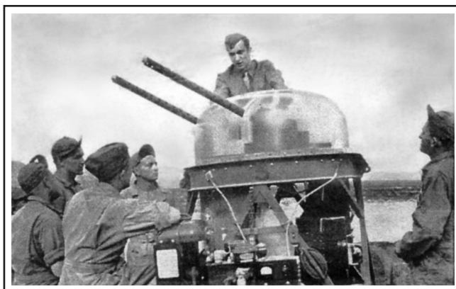
4. NEAR THE END OF THE FOUR WEEK COURSE the gunners learn how to operate power turrets, which have more elaborate sights than plain guns. The turret shown above is standard in B-24's and B-26's.
